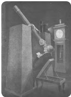
(top) Relic of a mural circle installed around 1840 and kept in service until 1857. Unfortunately it was scrapped around 1950. (left) An astronomer using a meridian transit telescope similar to that of the Royal Observatory. The telescope swung along the meridian and was used to time the precise moment at which a star passed the meridian due to the earth's rotation. This gave its right ascension, similar to geographic longitude. Note the regulator clock standing nearby so that the observer could hear and count its ticks. (right) A portable transit instrument used by Fallows before the Observatory was completed.
