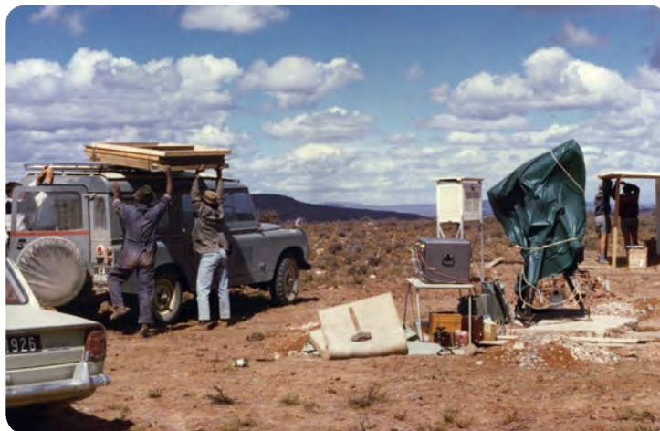
Site testing at Sutherland in the late 1960s. (left) Constructing the temporary observatory. (right) J Churms inspecting the double-beam telescope for monitoring the seeing quality.
