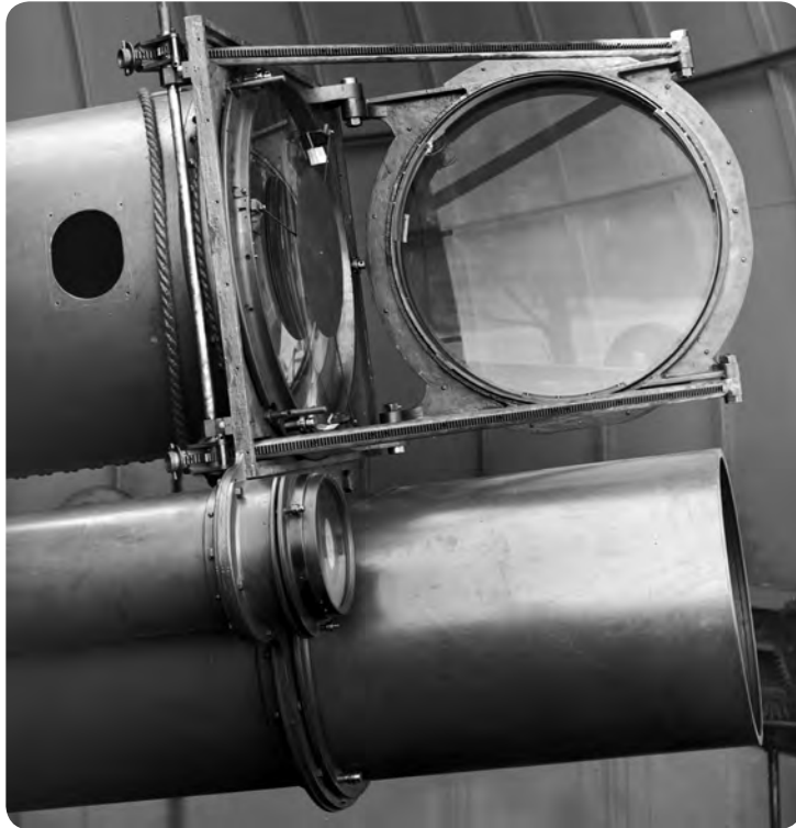
This telescope was fitted with many accessories. One of them was an “objective prism”, the largest ever made at the time, which fitted over the 24-inch lens and spread each star image out into a spectrum. Here it is seen folded away from the lens. The objective prism was used mainly during the first few years of this telescope.
