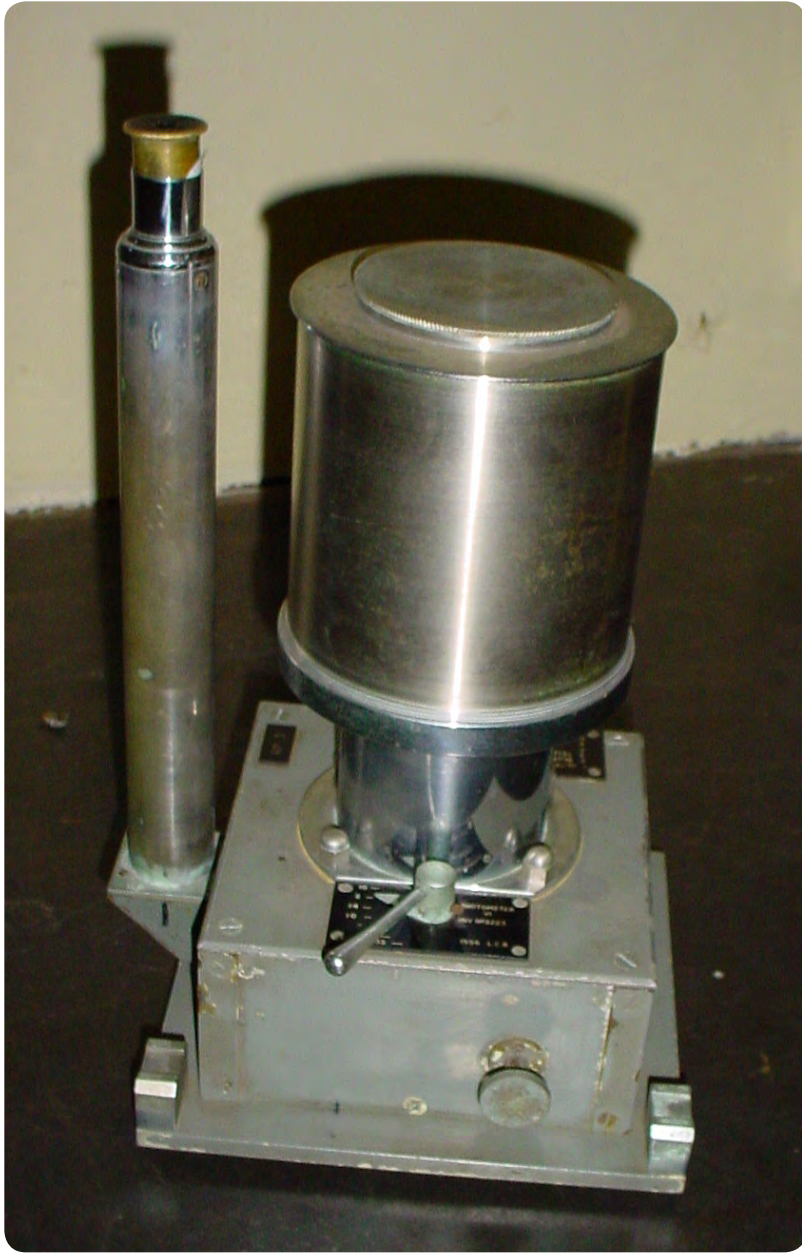
Photometer developed by AWJ Cousins and built at the Royal Observatory. It was used for precision photometry of southern bright stars, mainly on the 18-inch telescope.
