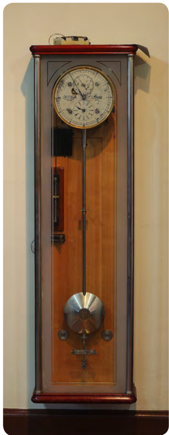
Riefler regulator clock from 1910 with electrical remontoire movement. Clocks of this kind were among the most accurate mechanical clocks ever built. This one was used at the Transvaal/Union/Republic Observatory.
