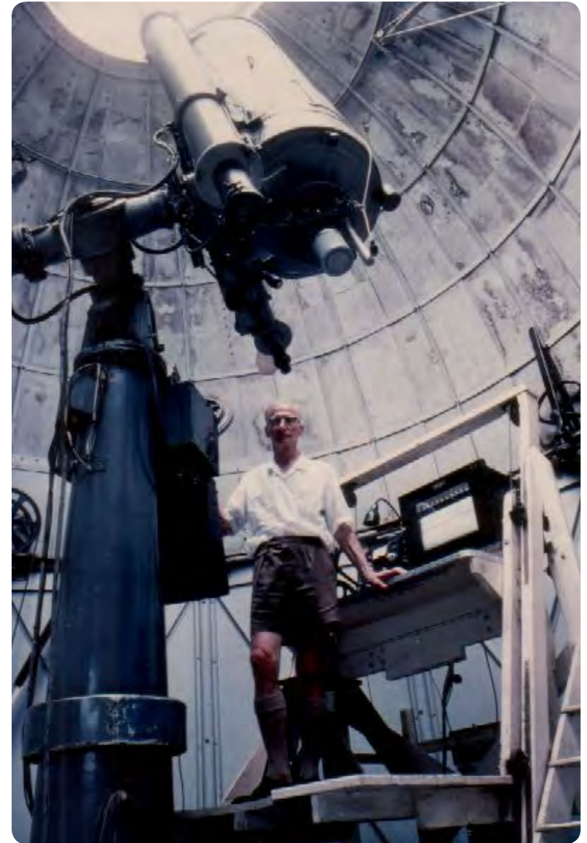
The 18-inch telescope on the former heliometer mount. A W J Cousins, the main user of this telescope, is seen on the observing platform, with his chart recorder in the background. The adjustable platform is an adaptation of the original Repsold observing chair.
